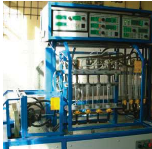
Photo. 22. Investigation of injectors with electronic control
