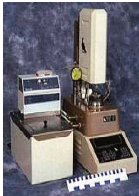
Photo. 12. Ravenfield HT/HS viscometer
