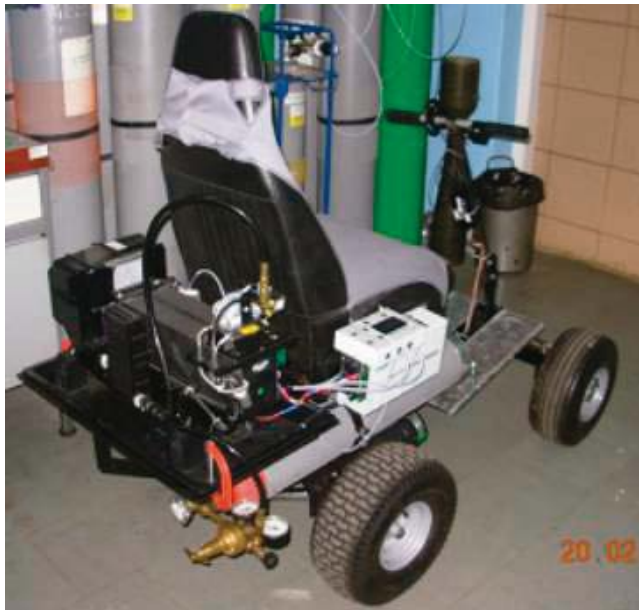
Photo. 21. Investigation of hybrid propulsion with fuel cell
