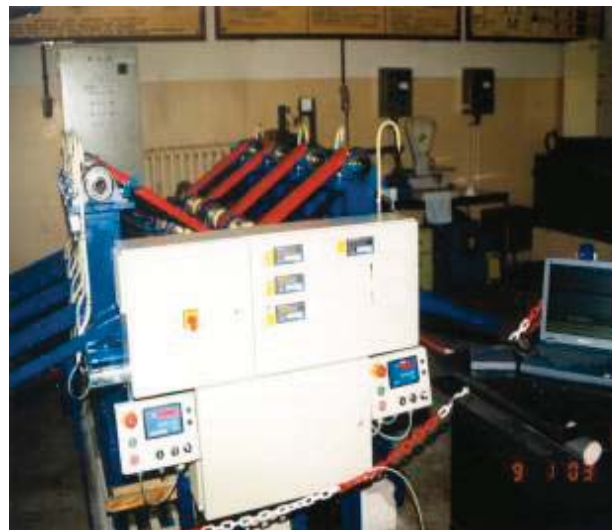
Photo. 10. Stand for investigations of self-lubricating bearings
